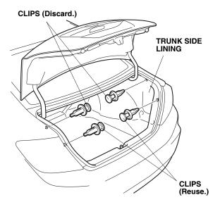
3. While wearing eye protection, enlarge the two clip holes shown to 9 mm. Remove any burrs, and apply touch-up paint to each hole. To prevent drilling through the inner panel, wrap tape around the drill bit 10 mm (0.4 in.) away from the tip.
